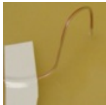
Fig 9. Thermocouple held in place using electrical tape prior to applying epoxy.
