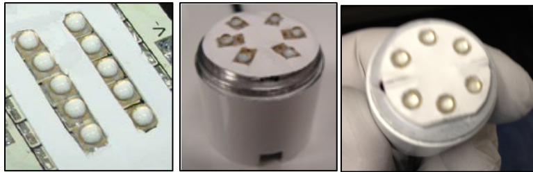
Fig 24. Mixing chamber material around LED arrays.
