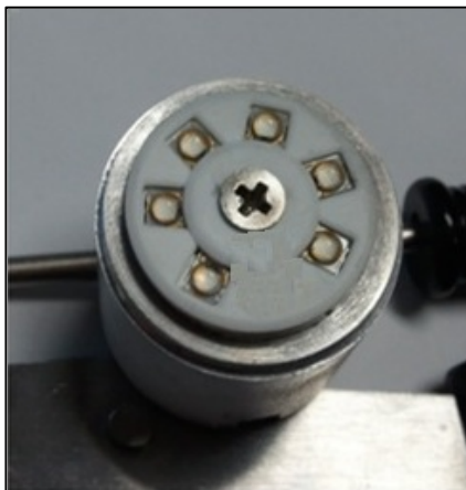
Fig 25. Flat head screw recommended.
